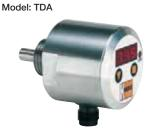
Measuring range: -58°F to +250°F p<sub>max</sub> 1,150 PSIG Connection: ½" NPT, ¾" NPT, G½, G¾ Output: 4-20 mA, 3-wire
