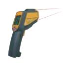
Measuring range: -76°F to +1,400 °F Laser sighting: single point and dual point Power: two AAA batteries Accuracy: ±2% of reading
